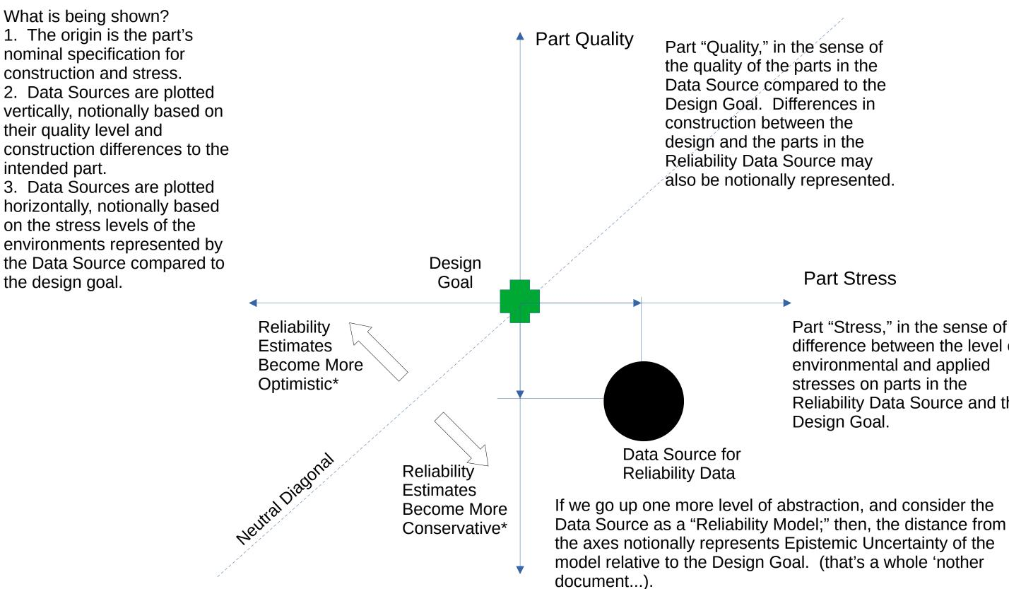
When a Reliability Data Source is Plotted, It has "Relativity" to the Design Goal \* "Optimistic" = Data Source would underestimate the failure rate of the part to be designed/estimated. "Conservative" = Data Source would overestimate the failure rate of the part to be designed/estimated.
