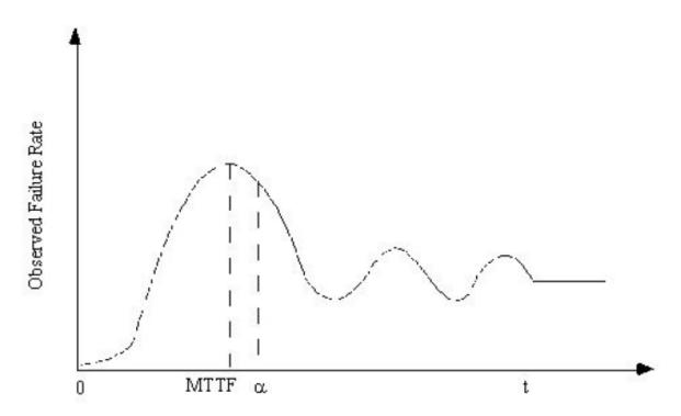
MTTF = Mean-Time-to-Failure, α = Weibull Characteristic Life
