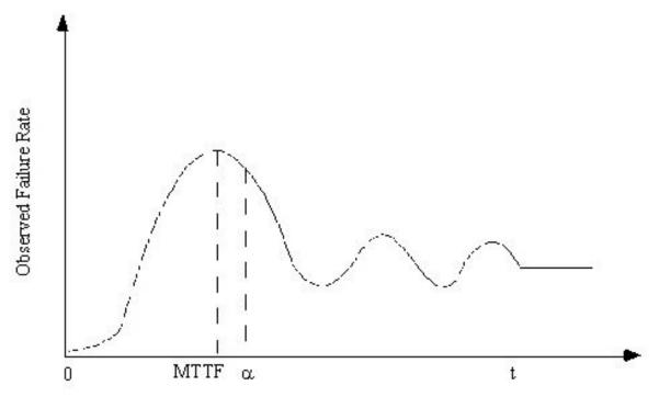
MTTF = Mean-Time-to-Failure,  $\alpha$  = Weibull Characteristic Life
